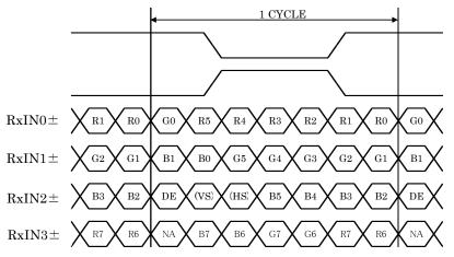
$\begin{array}{l} DE : DATA \ ENABLE \\ HS : H_{SYNC} \end{array}$
