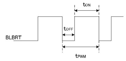
Please do not set toFF with 0  $\mu$  s < toFF < 1  $\mu$  s. In case of lower frequency, the deterioration of the display quality, flicker etc., may occur.
