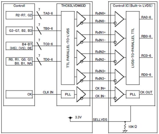
\*SELLVDS signal line has  $10 \text{ k} \Omega$  pulldown resister.
