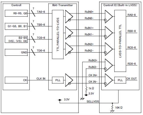
\*SELLVDS signal line has  $10 \text{ k} \Omega$  pulldown resister.
