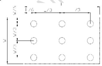
Lmax: The measured Maximum luminance of all measurement position.
