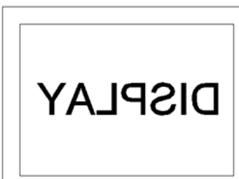
Fig. 9.10 Horizontal reverse (U/D: High; L/R: Low)
